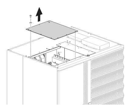
2 Top box: put it on the ground and remove cover, front panel and left side panel
