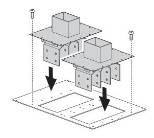
4 Top box: install top box without its cover onto the upper part of the UPS
