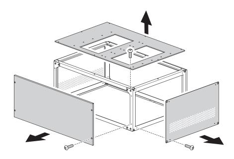
12 Side cabinet top box: put the upper cover on the ground and install the flanges (not supplied by Socomec)
