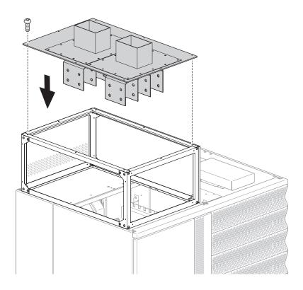
6 UPS system: internally connect the flanges to the UPS bus bars using the adapters supplied by Socomec
