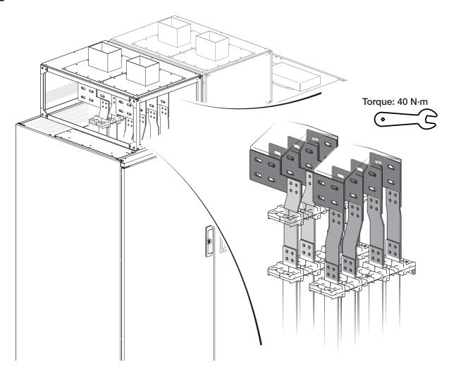
16 Reinstall the front and side panels of the top box and install the front panel of the side cabinet
