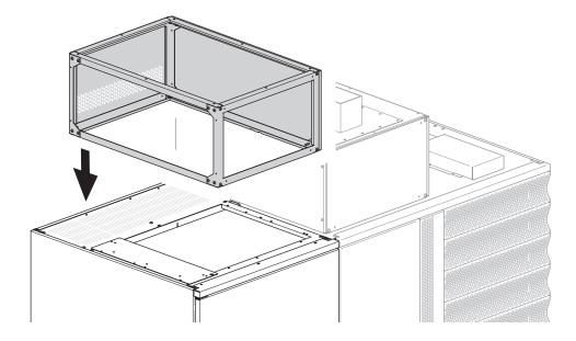
14 Side cabinet top box: install the upper cover with flanges onto the top box on the side cabinet
