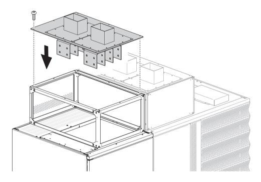
15 UPS system: internally connect the flanges to the UPS bus bars using the adapters supplied by Socomec
