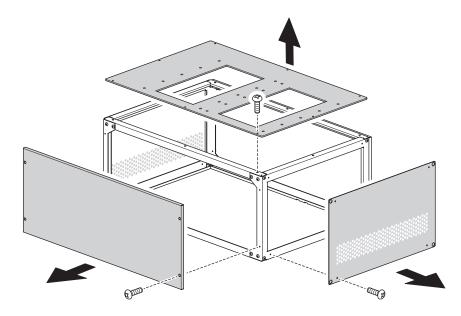
3 Top box: put the upper cover on the ground and install the flanges (not supplied by Socomec)
