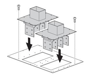
13 Side cabinet top box: install the top box without its cover onto the side cabinet
