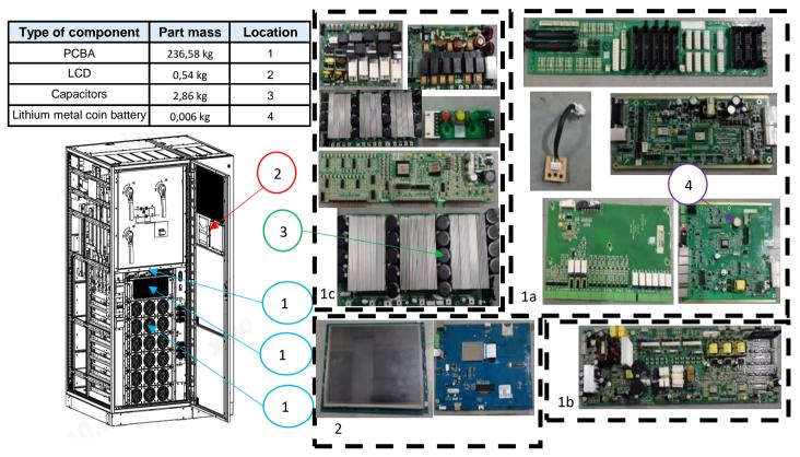
Waste of electrical and electronic equipment. Maintenance and disassembly should always be conducted by qualified personnel.
